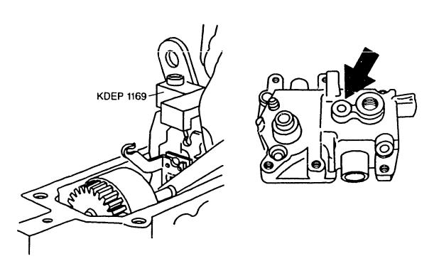
Mark control lever and shaft with respect to oneanother (arrows). Remove control lever and cylindrical helical coil spring. Remove cover fastening screws. If the rated-speed adjusting screw has to be removed, measure and note down screw-in depth beforehand. Raise cover and press through shaft in direction of inside of cover.
